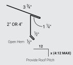
Profile Code: SB Detail Code: 03 Detail Num: D1F Profile Code: SB Detail Code: 03 Detail Num: D2 Girth Num: 10.0"
